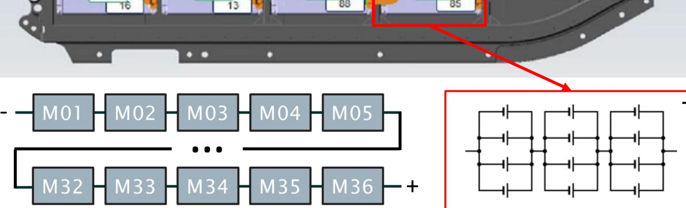
The pack consists of 36 battery modules connected in series to form a single string. Each module is comprised of 12, 60 Ah lithium nickel manganese cobalt oxide (Li-NMC) cells in a 4-parallel 3-series arrangement.
