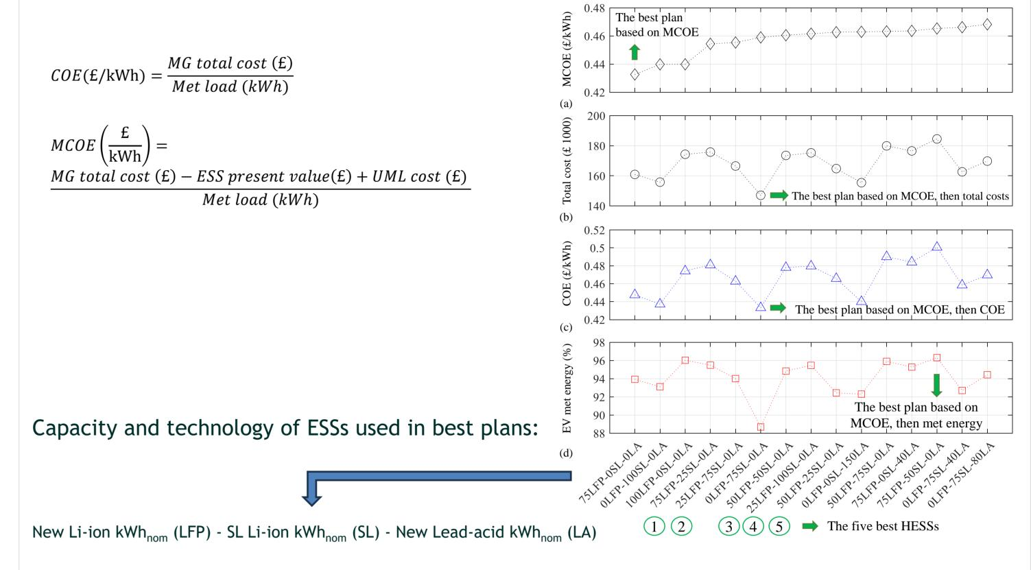
where the present value of energy storage systems (ESSs) and the virtual cost of unmet energy of the electric vehicle (EV) charging station are considered.
